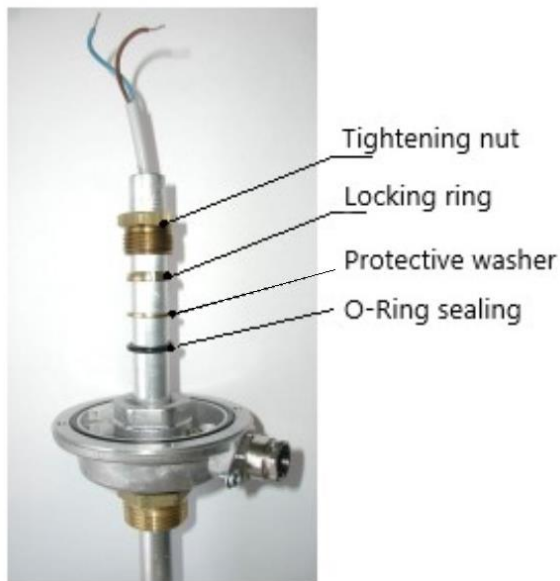
Figure 5. Sensor pipe mounting
